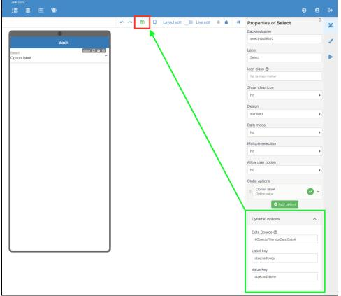
13. Open mobile app and check the result (in this picture - Option label is from Static options in that component)
